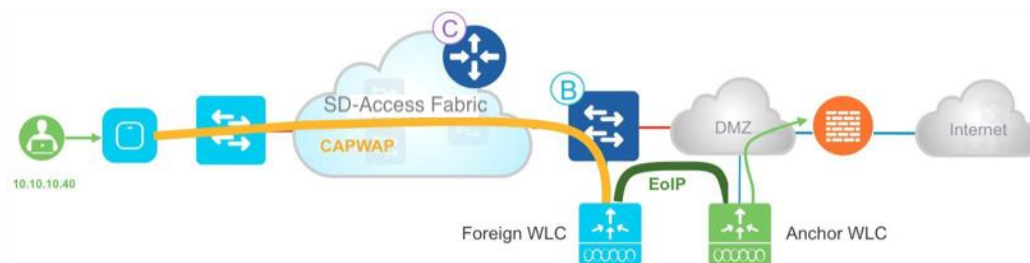
Figure 40. OTT solution using a guest anchor controller
