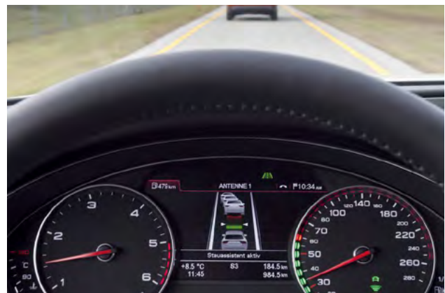
Figure 6: Audi's Adaptive Cruise Control helps to keep a safe distance from the vehicle in front; Source: Hearst Communications
