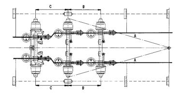
Semi-trailers with trailing steering axle Distance A, B, C max. permissible deviation 1.0 mm Toe setting  $\pm$  12' =  $\pm$  3.0 mm/m Camber  $\pm$  12' (values apply to unloaded vehicle)
