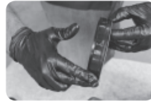
Lightly lubricate the O.D. and I.D. with the fluid being retained.
