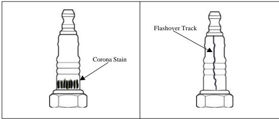
You may never see Corona; however, it may leave a telltale, non-conductive, yellow or brown stain around the insulator base below the plug wire boot near the top of the shell. This stain should not be interpreted as leakage between the shell and insulator.
