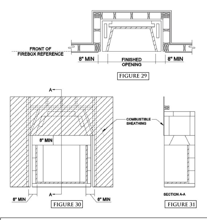
Combustible sheathings must be held a minimum of 8" away from each side and a minimum of 8" above the top of the finished fireplace opening. (Figures 29 & 30)
