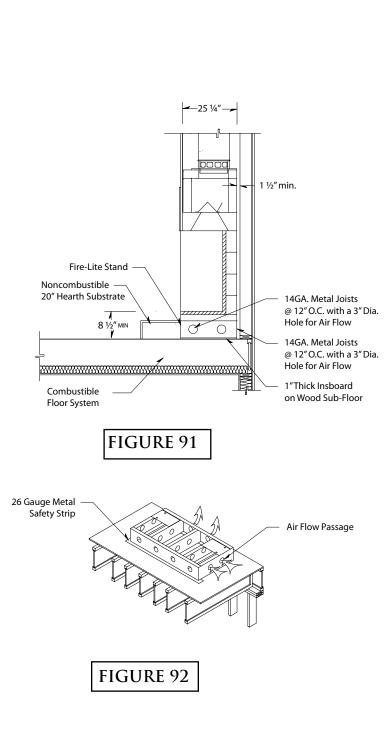
The noncombustible raised platform must be set with a minimum one and one half inch (1-1/2") clearance to the wall directly behind the Fire-Lite assembly.
