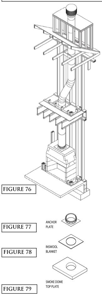
STANDARD fireplaces are tested and listed for use with factory-built metal, Class "A" (solid fuel) chimneys as an option. Any Class "A" or UL 103 listed metal chimney system is accetable for use on an Isokern system. (Figure 76)
