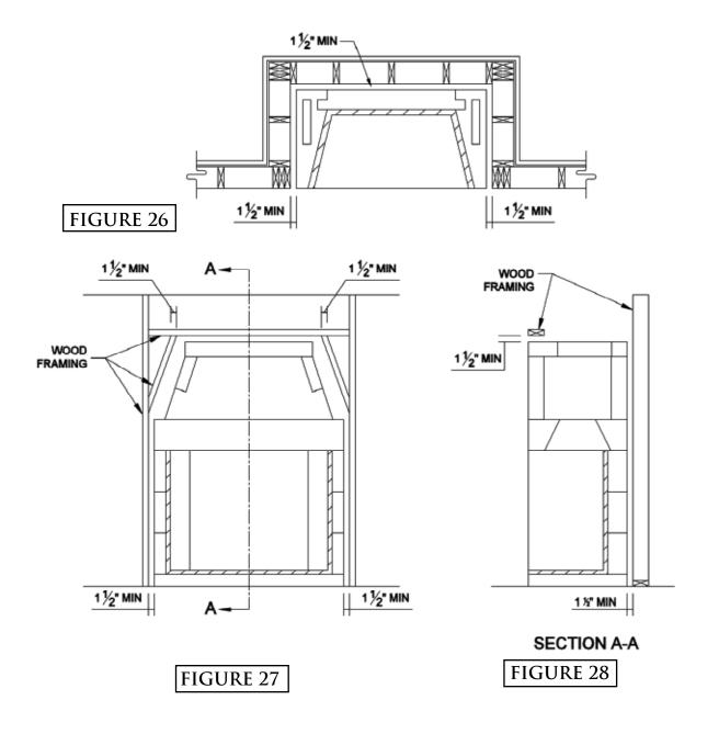
The STANDARD Series Isokern fireplace is tested and listed for 1 1/2" clearance to un-insulated wood framing material at the firebox sides, back and at the smoke dome front, sides and back. However installation and use practices that are beyond the control of the manufacturer\* can create situations where a zero clearance installation can jeopardize the safety of combustibles in contact with the Isokern surfaces resulting in fire damage to property, personal injury or loss of life.
