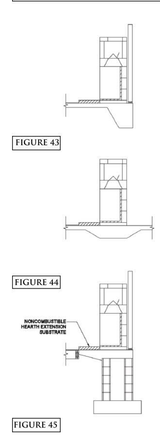
The STANDARD fireplace is not rated for installation on a combustible floor system unless used in the Fire-Lite application (see Pages 47-55). STANDARD fireplaces must be built upon a concrete support slab with no wood underpinnings. Proper reinforced concrete support slab for STANDARD installations may include the following types:
