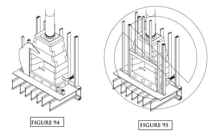
STANDARD Fire-Lite Series fireplaces are designed to be installed so that the rough front face of the firebox and smoke dome sit flush to the room face of the rough framing members that create the room wall finish. (Figure 94)
