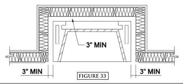
The STANDARD Series firebox back wall, the firebox side walls and the smoke dome back require 1-1/2" clearance. (Figure 32) Keep all insulation and vapor barriers a minimum of 3" away from all Isokern fireplace surfaces.
