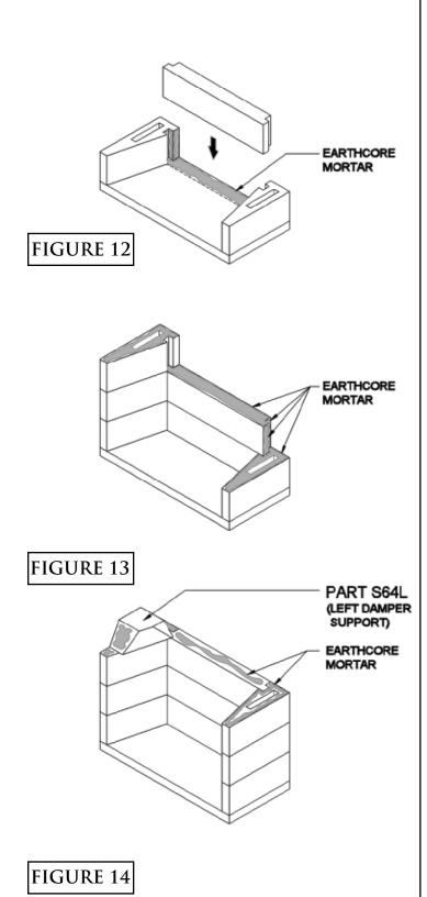
Step 3: Continue assembly of the second, third and fourth courses of the firebox side wall and back wall. Apply mortar to the top of each layer of wall components, set the next course above into place. Be sure to mortar all vertical joints of the side wall to back wall connection when setting each component to its mate. (Figure 13)
