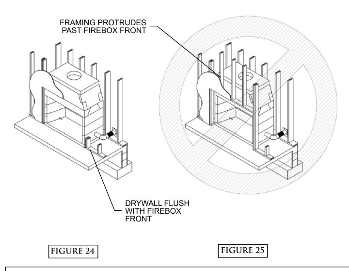
STANDARD Series fireplaces are designed to be installed so that the rough front face of the firebox and smoke dome sit flush to the room face of the rough framing members that create the room wall finish. (Figure 24)
