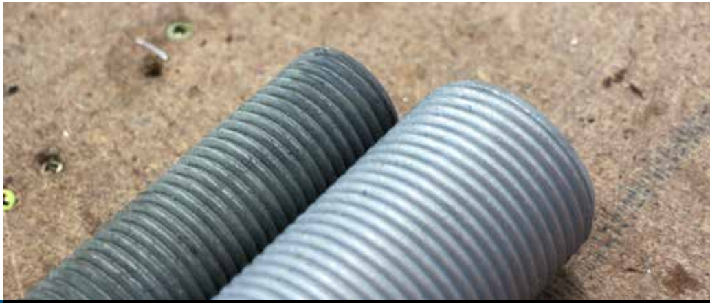
HDG (left) compared with Mechanical Galvanised (right)
