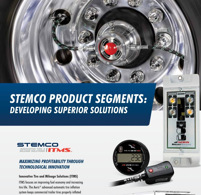
ITMS focuses on improving fuel economy and increasing tire life. The Aeris® advanced automatic tire inflation system keeps commercial trailer tires properly inflated using air pressure from the trailer's braking system.
