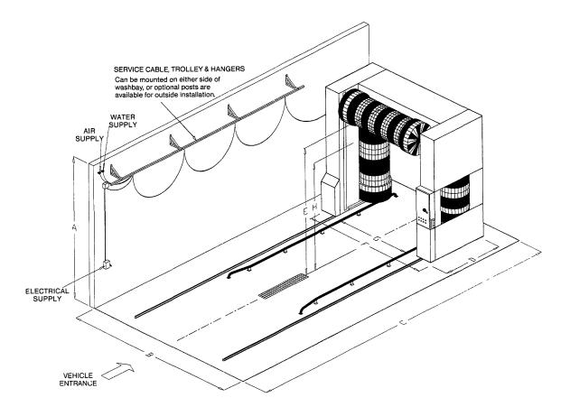
FIGURE 5 Schematic drawing of a typical gantry washing system. (Courtesy of SSI Corp.)
