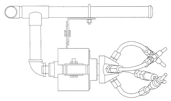
FIGURE 6 Schematic drawing of a high-pressure spinner wheel washer. (Courtesy of SSI Corp.)
