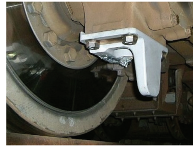
Fig. 12 L-shaped guide to prevent deviation from rails
