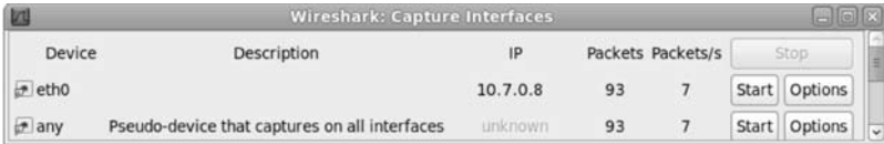
Figure 2.10. Wireshark capture interfaces window
