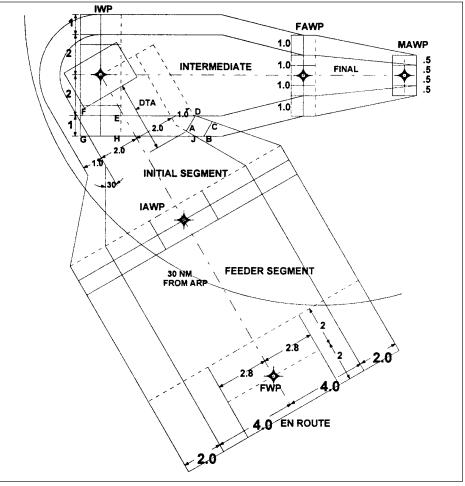
The segments of a GPS instrument approach from FAA Order 8260.38A. Note the final approach segment primary area is only 0.5 nm either side of centerline, which is closer to ILS tolerances than the typical non-precision approach. Abbreviations: ARP - Airport Reference Point, FWP - Feeder Waypoint, IAWP - Initial Approach Waypoint, IWP - Intermediate Waypoint, FAWP - Final Approach Waypoint, MAWP - Missed Approach Waypoint.
