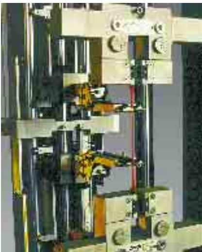
The mechanical long-stroke-extensometer is designed for measurements on rubber and plastics.
