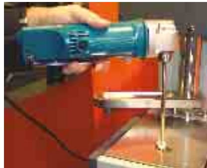
Cleaning of the extrusion barrel with an angle drill
