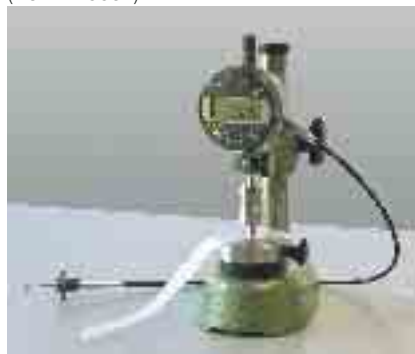
Dead weight thickness gauge providing a constant measuring force (DM-THICKGA.00 + DM-PLASTFOI.S00)
