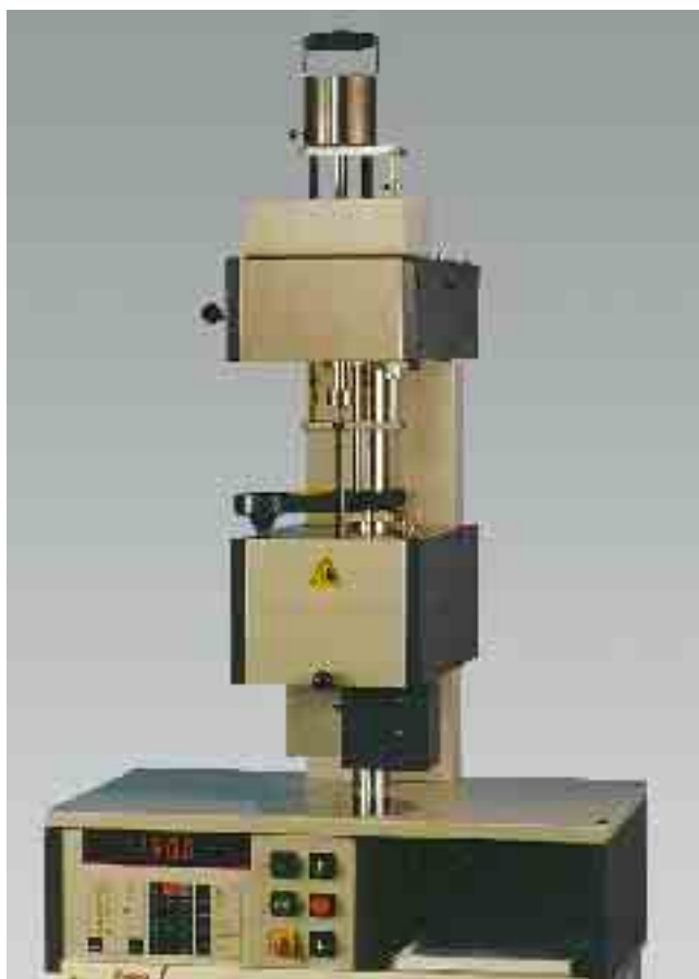
Plastometer Zwick 4106 including piston travel measurement and weight release system for MFR and MVR determination
