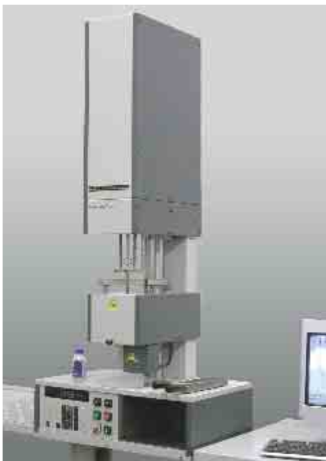
Plastometer Zwick 4106 including automatic, freely programmable weight change unit.
