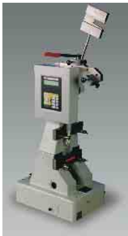
Pendulum impact tester Zwick 5113 (50 Joule) with digital display
