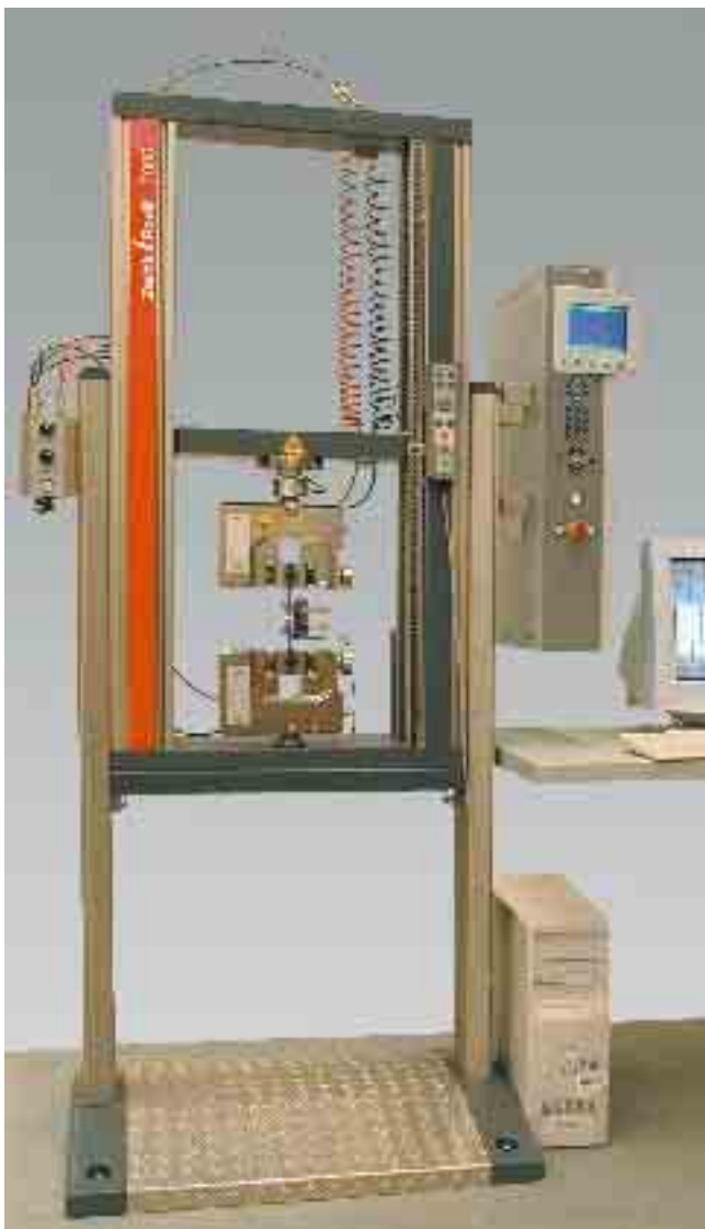
Materials testing machine Z05 for the determination of tensile properties of plastics.
