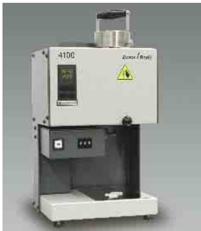
Plastometer type Zwick 4100 for measurements acc. to method A
