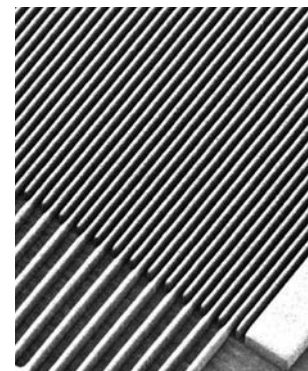
Design L/S=5/5 \mu\text{m} with PF-EL SP (Exposure Stepper)
