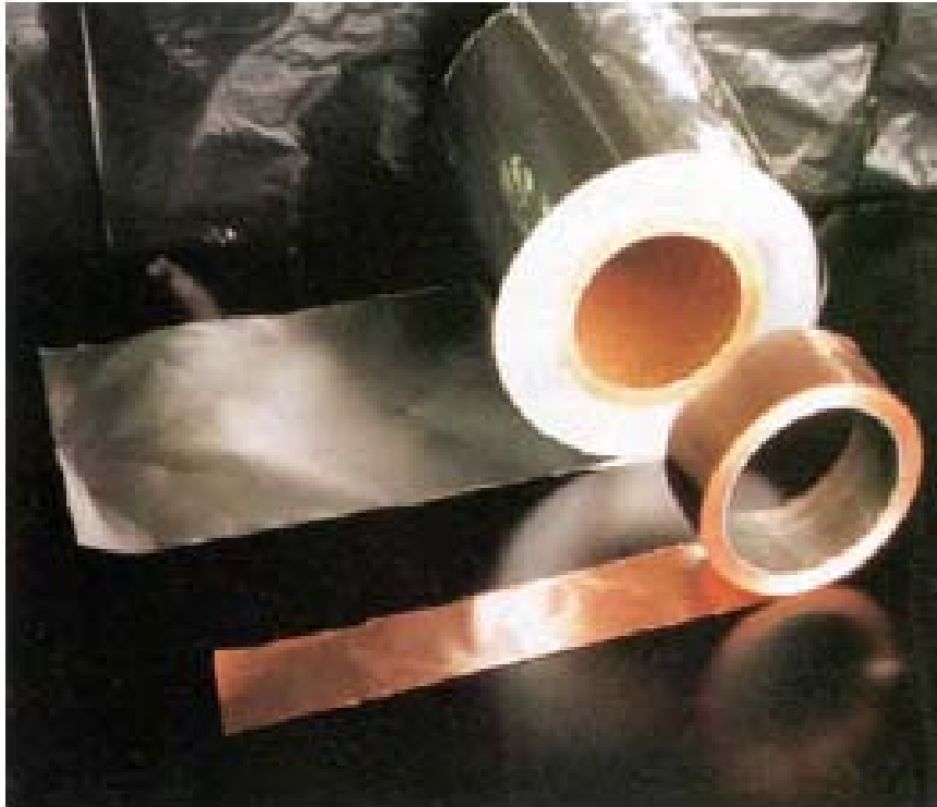
Current Collectors Aluminum foil (Cathode) 20 \mu m Copper foil (Anode) 14 \mu m
