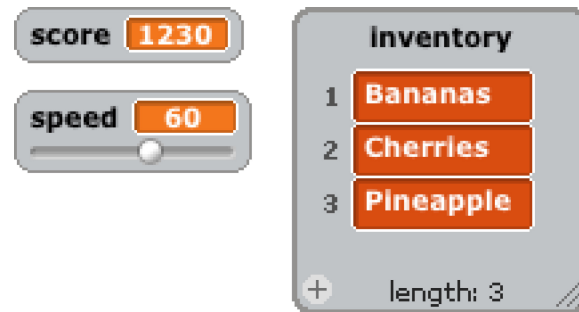
Fig. 5. Scratch variable monitors (left) and list monitor (right). The optional slider allows a variable to be used as a control.
