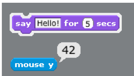
Fig. 3. Blocks can be tested simply by clicking on them. A white border indicates that a block or stack is running. Function blocks show their output in a talk bubble.
