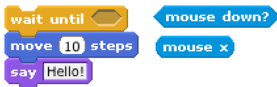
Fig. 6. Shapes indicate type. On the left, command blocks with parameter slots for boolean, number, and string parameters. On the right, boolean and number function blocks.
