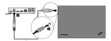
Figure 3. Connecting the ultra dock to the power supply and notebook computer
