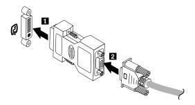
Figure 9. Using the DVI-I to VGA adapter
