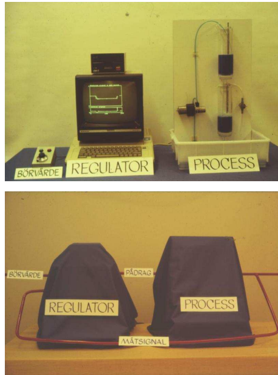
Figure 6.9: Illustrates the process of information hiding used to obtain a block diagram. The top figure is a picture of the physical system, the middle figure is obtained by hiding many details about the system and the bottom figure is the block diagram.
