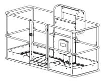
A Tri-entry platform with three sliding mid-rails
