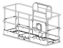
▲ Tri-entry platform with two sliding mid-rails and center mounted swing gate
