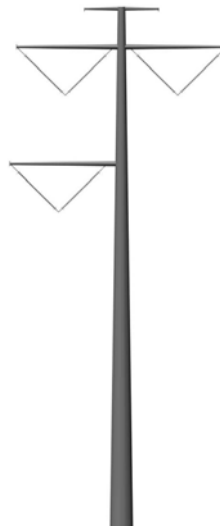
500-kV single-circuit TSP
