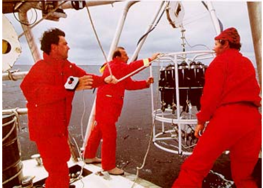
SBE 9plus underwater unit mounted to Carousel
