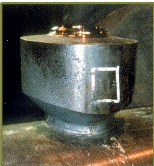
Fig 5: Thick-walled pipe connection of a live-steam pipe of P91
