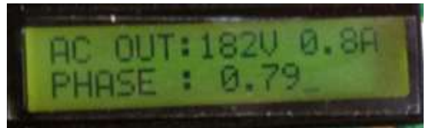
Fig5. Result of resistive load
