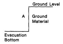
SIDE A: If examination of the ground indicated hazardous ground movement may be expected Side A shall be cut to the angle of repose of a supporting system shall be provided.
