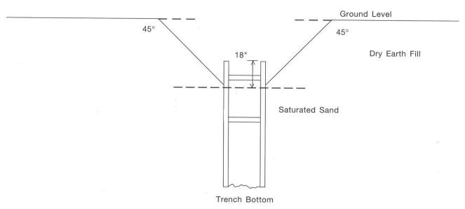
If the bottom of the trench extends into saturated sand, soft clay, or organic soil under a fill, a trench supporting system should be used to provide protection below the fill.
