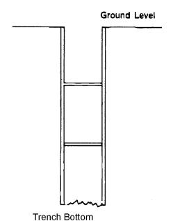
A trench support system shall be designed by a qualified employee knowledgeable in the field. The arrangement of stringers, struts, and braces should be a designated by the plans.
