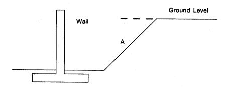
Side A: Side A should be cut to the angle of repose or a supporting system provided.
