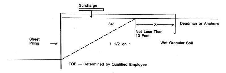
The design of the supporting system should take into consideration any surcharge, such as, stockpiled material, equipment, or hydrostatic pressure that must be supported by the system.
