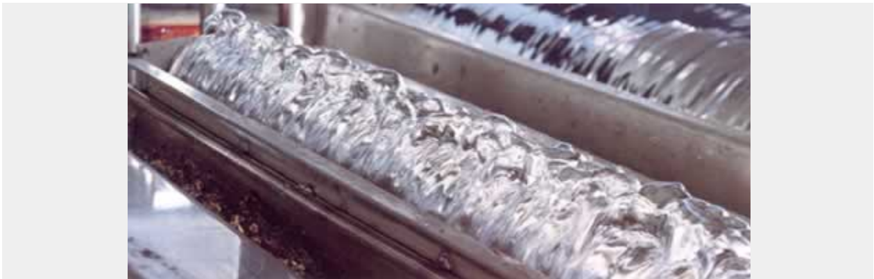
Figure 12: Close-up of turbulent chip wave
