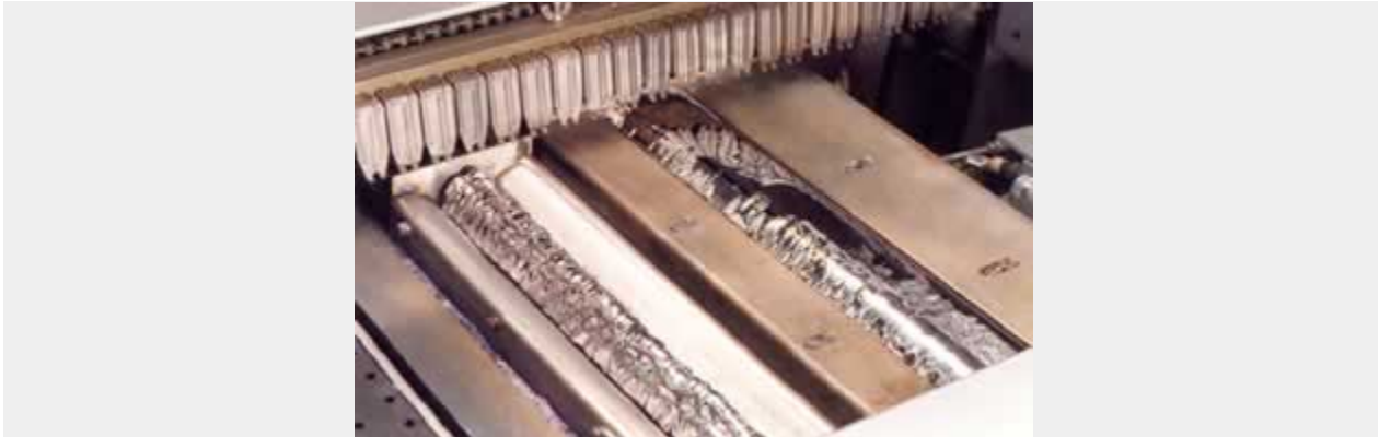
Figure 11: Double wave system: the 'chip' wave is on the left
